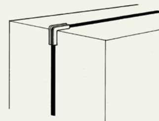
[ Improved cargo packing (L-shaped ironware used) ]
