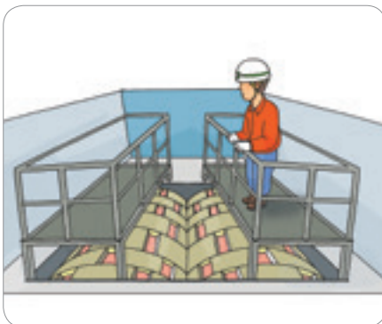
Safety Railings around Scaffolding
