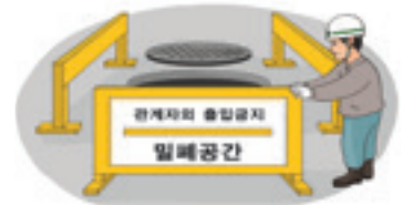
Authorized Personnel Only Enclosed Space
